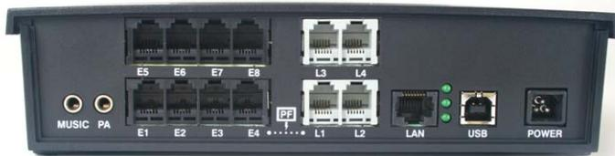
The PF box between E4 and L1/L2 represents power failure support. In the event of a power failure or loss of power to TalkSwitch, extension port E4 is able to receive and make calls on Line 1.
